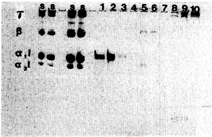
Fig. 3. SDS-polyacrylamide gel analysis of fractions collected after HPLC of denatured bovine type I collagen chains. HPLC was carried out with 0.02 M ammonium bicarbonate in solvent A (TFA-water), see Fig. 2c. S = Standard type I collagen. Note that \alpha_1 chains appear in fractions 1-3, \alpha_2 chains and \beta components in fractions 5 and 6 and \gamma components in fractions 8-10.
